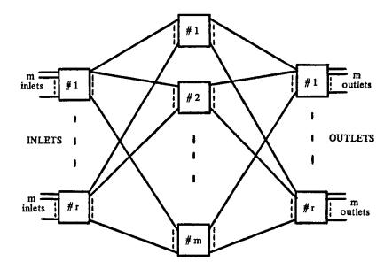
Each square box represents a switching unit for which any of the possible permutations of connecting its local inlets to its local outlets is possible. The problem is to show that this network is rearrangeable, i.e., given any set of calls in progress and any pair of idle terminals, the existing calls can be reassigned new routes (if necessary) so as to make it possible to connect the idle pair. How is the reassignment made so as to change the minimum number of existing calls? (cf. [Ben].)
