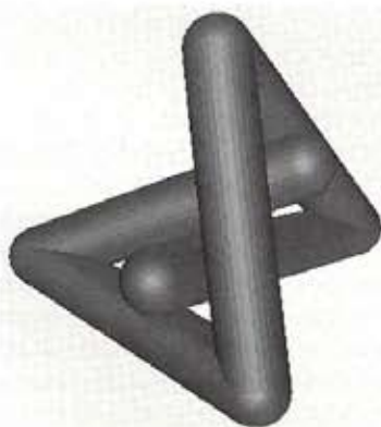
A chain of five equal-length cylindrical links, which is apparently locked even with all universal joints.
