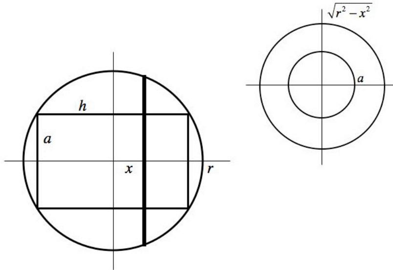
Consider a slice through the napkin ring a distance  $x$  from the origin, where  $-h \leq x \leq h$ , shown as a dark vertical line in the cross-section diagram to the left. Face on, this section will be an annulus, shown in the diagram on the right. The radius of the inner boundary of the annulus is  $a$ , the diameter of the cylinder. The radius of the outer boundary is, by Pythagoras' theorem,  $\sqrt{r^2 - x^2}$ . The area of the annulus is thus:
