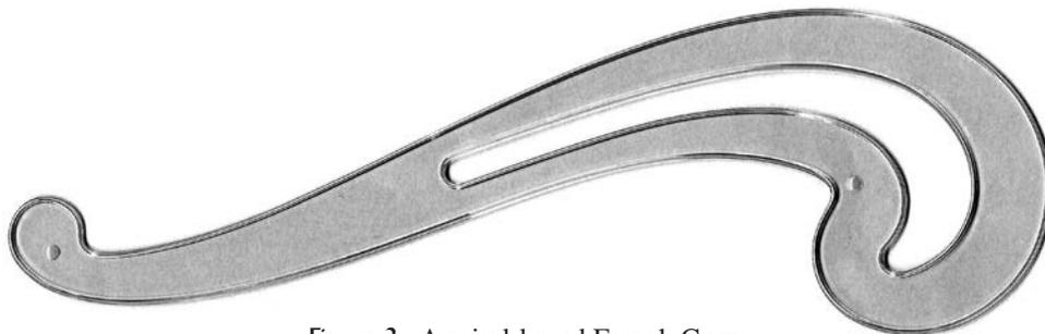
Figure 3. A spiral-based French Curve
