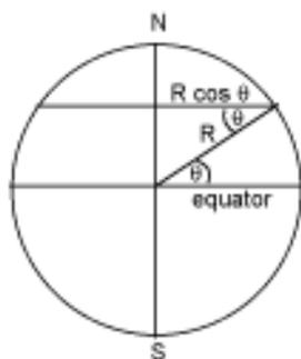
**Figure 1.** A cross-section shows why the distance involved in traveling around the Earth at a given latitude is proportional to the cosine of that latitude.
